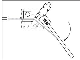
Figure 14. Bending workpiece.
